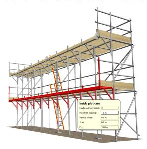
Inside standards have been added at a spacing of 1m to support the extra brackets.
