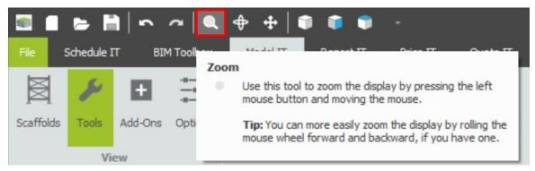
Click on the **Zoom** tool to activate it; then zoom in and out by moving the mouse to the 3D view, pressing and holding the left mouse button, and moving the mouse up and down.
