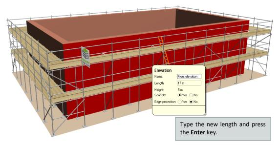
The height of the scaffold can be modified in the same way. Either drag the top of the building to the required height or move the mouse pointer to the top of the building and type the new height.
