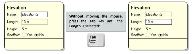
Press the **Tab** key so that **Length** is highlighted. Type in the new length and press the **Enter** key:
