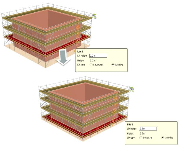
Alternatively, you can type the lift height directly in the same way as the elevation lengths. Place the mouse pointer over the bottom lift, type "0.5" and press **Enter**.
