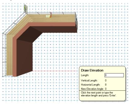
As the mouse is moved the **Length** field is updated so that you can measure the length of each elevation as you draw.
