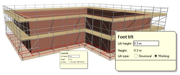
For most scaffolding systems, the height of the base jacks can be set even when a foot lift is not present, by dragging the **foot lift grips**:
