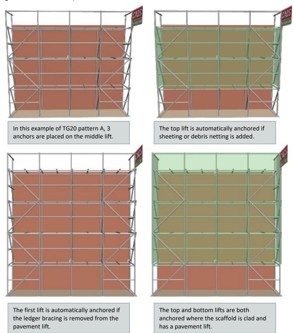
The anchor patterns for system scaffolds follow the rules from the manufacturer's user manuals. Some systems include additional anchor patterns which have been requested.
