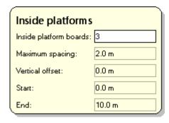
You can change the spacing of the brackets (on a tube-and-fitting scaffold) by moving the mouse over the platform, pressing the **Tab** key until the **Maximum spacing** field is highlighted, and entering the new maximum spacing in metres. If the spacing of the brackets is less than the spacing of the standards then new intermediate standards will be added where required.
