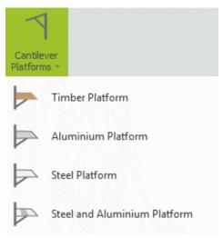
Cantilever platforms are applied to boarded lifts by selecting the required deck type and clicking on the lifts that you wish to apply the platforms to.
