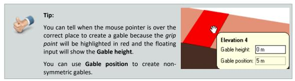
As you create the gable end a symmetrical gable end is created on the opposite elevation, if present. You can prevent this from happening by holding the **Ctrl** key while dragging the mouse.
