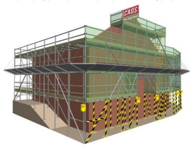
SMART Estimator **Model IT** now supports tube-and-fitting scaffolding and system scaffolding, with the present version supporting the Cuplok, Kwikstage, Layher Allround, HAKI Universal and Frame Scaffolding systems.
