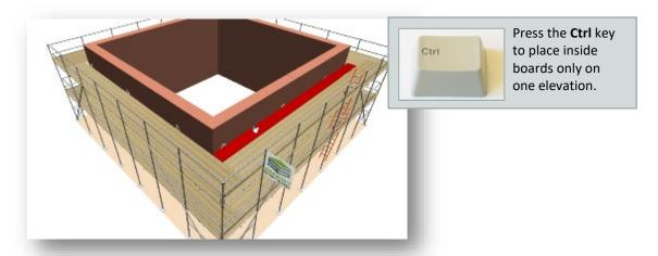
If you prefer you can also edit the inside boards using the keyboard – move the mouse to the gap between the scaffold and the building, enter the number of inside boards, and press **Enter**:
