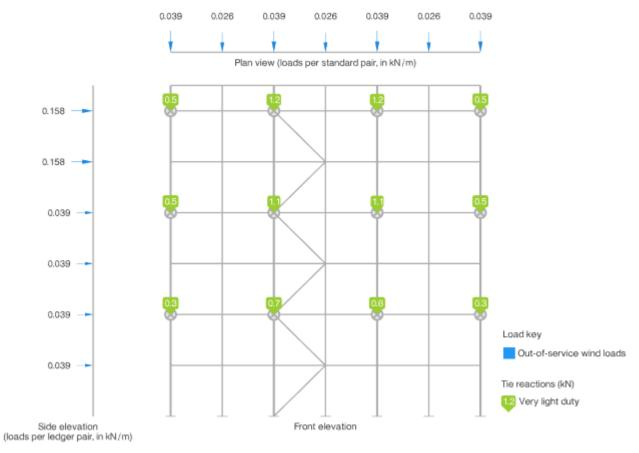
The analytical model is shown for the load combination which produces the maximum tie duty: 3 - Out-of-service wind loads.
