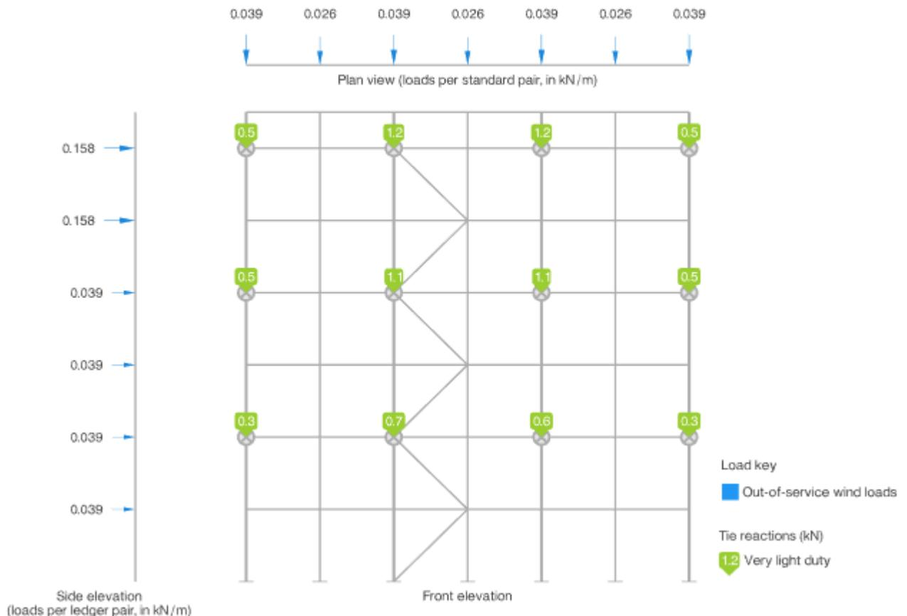
The analytical model is shown for the load combination which produces the maximum tie duty: 3 - Out-of-service wind loads.
